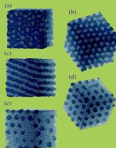
IRG 1: Engineering particle interactions in nanocomposite materials enables realization of dramatically different morphologies.
