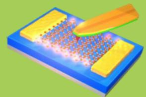
IRG 2: Microwave impedance microscopy enables characterization of electrical conductivity in advanced transistors at the nanoscale.
