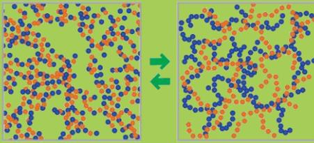
**IRG 1, Reconfigurable Porous Nanoparticle Networks**, addresses multifunctional, reconfigurable networks of nanoparticles, polymers, and organic molecules that respond to a range of external stimuli. Controlled assembly and reconfiguration of nanoparticles connected by molecular linkers enables unique optical, chemical, or biological materials functionality.
