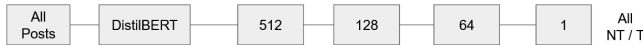
Figure 1: Architecture for Single Task, where all posts are passed through a neural network and get classified as toxic vs. non-toxic.
